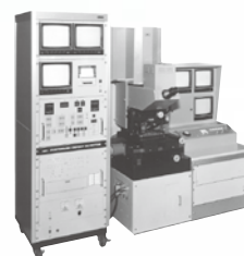
LSI photomask inspection system in 1976 (Winner of “Ten Best New Products Award” from Nikkan Kogyo Shimbum)
