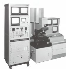
LSI photomask inspection system in 1976 (Winner of "Ten Best New Products Award" from Nikkan Kogyo Shimben)
